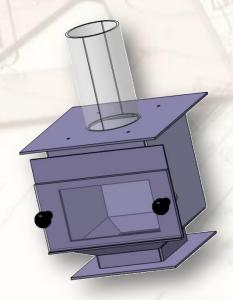
The picture on the right, is a picture of the Housing Magnet. Housing Magnet is a place holder or magnets home that used to filter the seeds (grains) plastic that will go into plastic injection machine.
